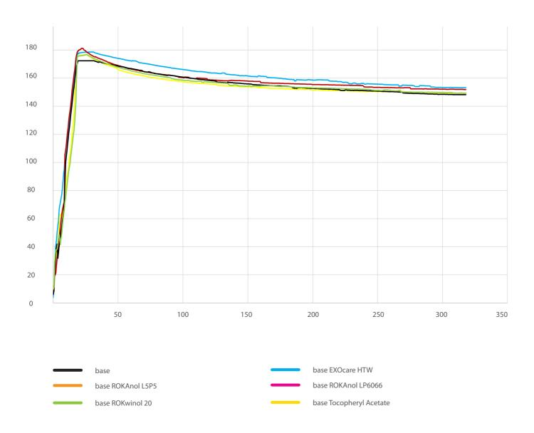
DFA100 KRÜSS foam analyzer Investigation of the foam formation and foam disappearance process for 1.0% of active substance (SA) of the formulation diluted in tap water at 20°C.
