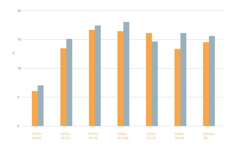
The cleaning process is described by the dL parameter in accordance with the CIE LAB method. The standard is the soiled fabric, so the higher the value of the dL parameter, the better the tested fabric is cleaned.
