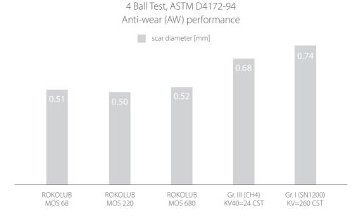
load = 40 kg, T = 75 C, speed = 1200 rpm, time = 60 min
