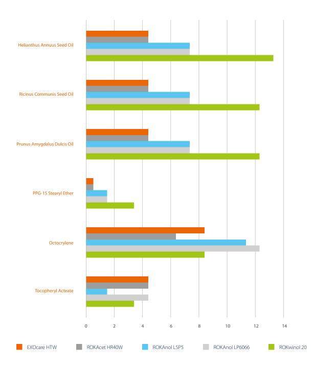
Solubilization test determining the amount of solubilizer needed to introduce 0.5% of water-insoluble components to obtain a clear mixture.
