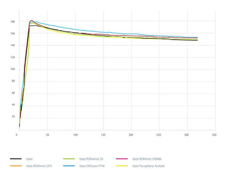
DFA100 KRÜSS foam analyzer Investigation of the foam formation and foam disappearance process for 1.0% of active substance (SA) of the formulation diluted in tap water at 20°C.
