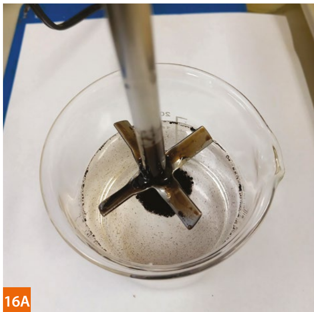
Pic. 16A/16B Degreasing capability. Dynamic test, ROKAnol ID8 (concentration of 2.0 g/l) after 2 min and 5 min
