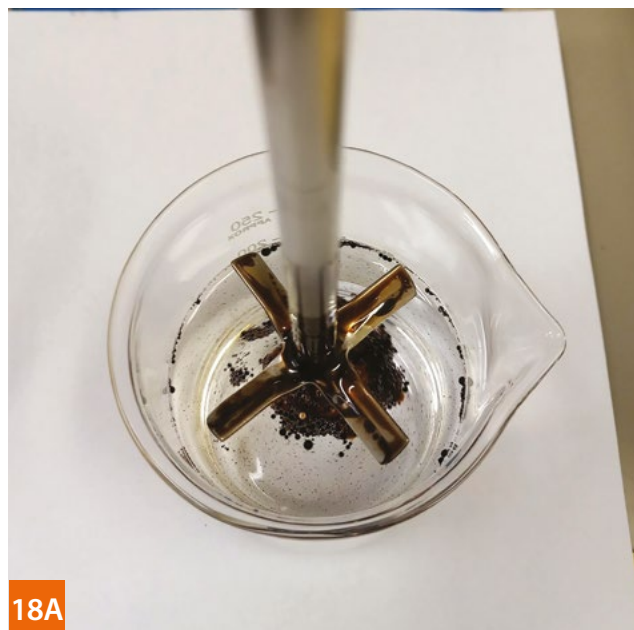
Pic. 18A/18B Degreasing capability. Dynamic test, ROKAnol ID11 (concentration of 2.0 g/l) after 2 min and 5 min
