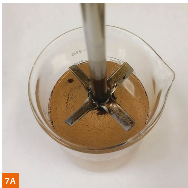
Pic. 7A/7B Degreasing capability. Dynamic test, ROKAnol ID5W (concentration of 5.0 g/l) after 2 min and 5 min
