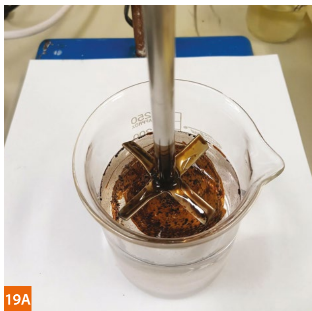
Pic. 19A/19B Degreasing capability. Dynamic test, ROKAnol ID11 (concentration of 5.0 g/l) after 2 min and 5 min
