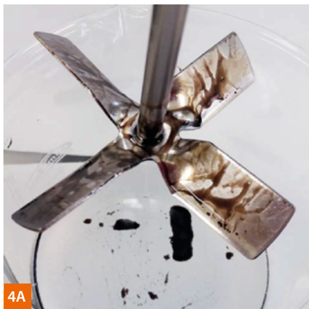
Pic. 4A/4B Degreasing capability. Dynamic test, ROKAnol GT6, after 2 min and 5 min.
