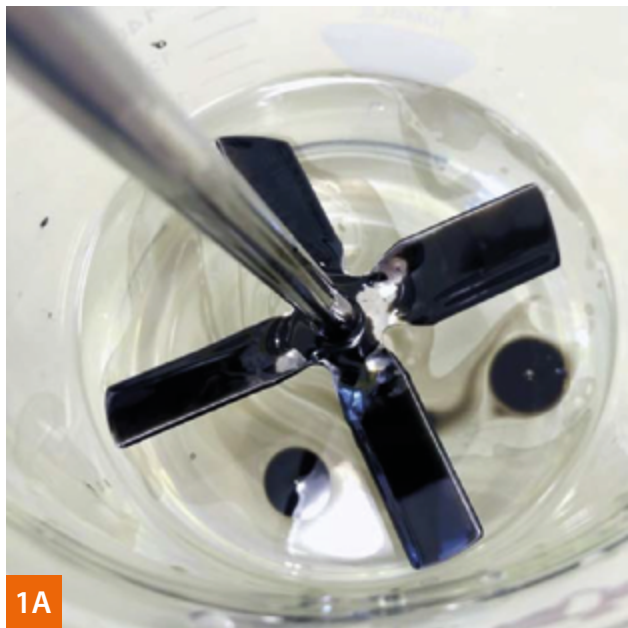
Pic. 1A/1B Degreasing capability. Dynamic test, demineralized water, after 2 min and 5 min.
