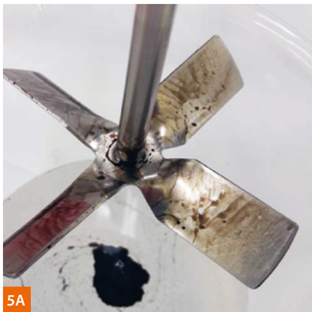
Pic. 5A/5B Degreasing capability. Dynamic test, ROKAnol GT7, after 2 min and 5 min.
