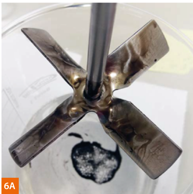
Pic. 6A/6B Degreasing capability. Dynamic test, ROKAnol GT8, after 2 min and 5 min.
