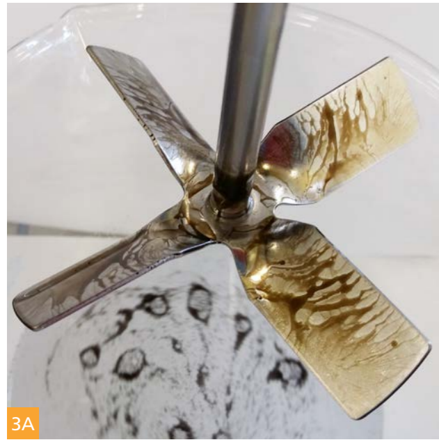
Pic. 3A/3B Degreasing capability. Dynamic test, ROKAnol GT5, after 2 min and 5 min.
