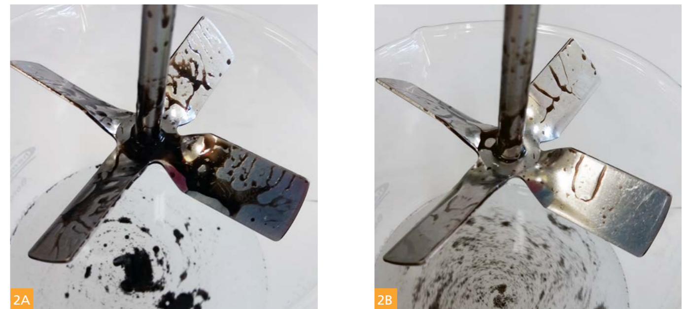
Pic. 2A/2B Degreasing capability. Dynamic test, ROKAnol GT3, after 2 min and 5 min.
