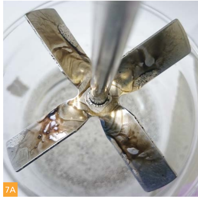
Pic. 7A/7B Degreasing capability. Dynamic test, ROKAnol GT9, after 2 min and 5 min.
