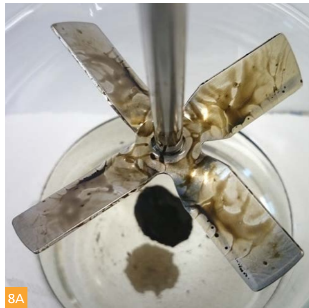
Pic. 8A/8B Degreasing capability. Dynamic test, ROKAnol GT10, after 2 min and 5 min.
